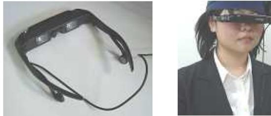
**Fig. 1.** An HMD (iWear AV920, Vuzix Corporation; 640×480dot) used in the present experiment
