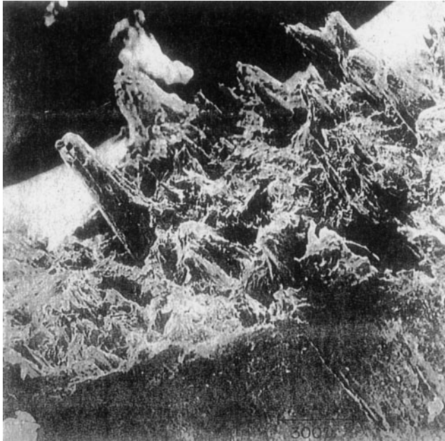
FIG. 4. A typical fracture surface of compact lamellar bone of the beef femur fractured at low strain rate (after Piekarski 20 ).
