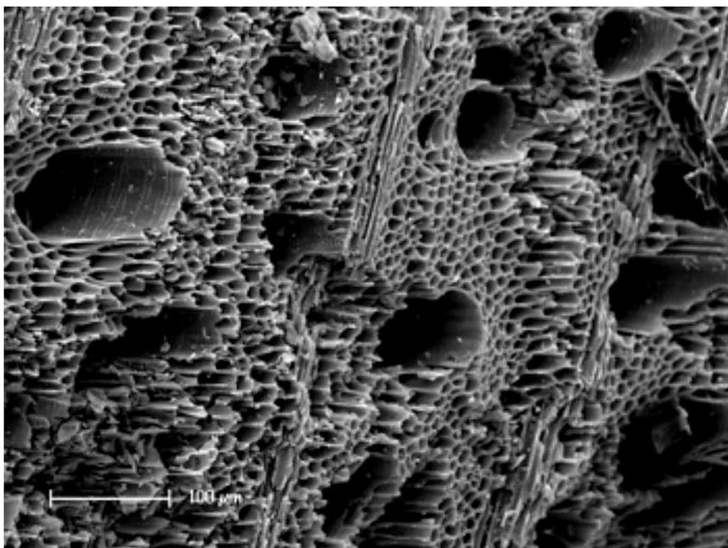
**Figure 1.** Biochar under a microscope, Brownsort, UK Biochar Research Centre.
