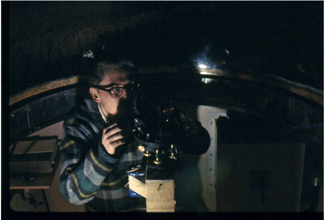
Top: Bob Geissel tracking a balloon in flight in order to compute the wind speed and direction by triangulation
