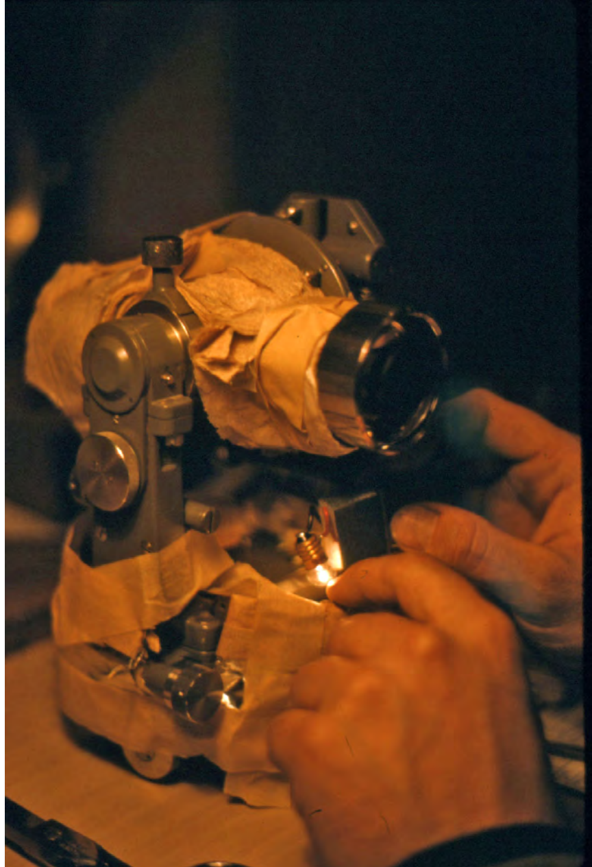
Keeping a transit warm by packing it with hot activated pibal light batteries
