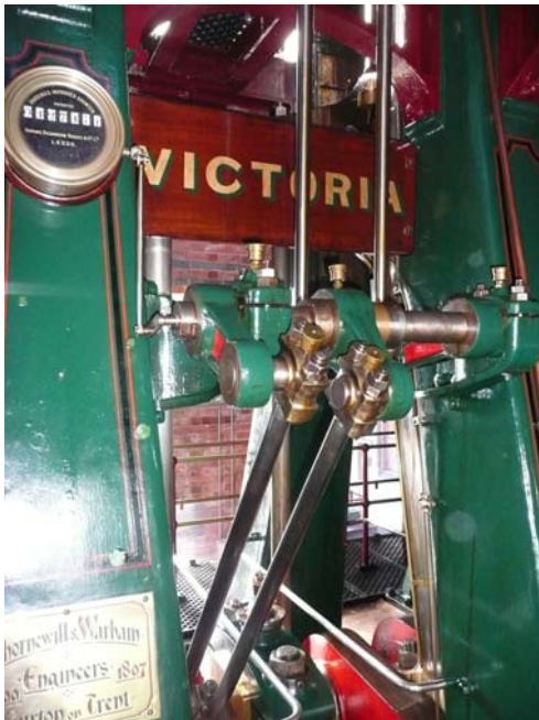
Fig. 2. Vertical triple expansion steam engine at The Bratch (courtesy of Friends of The Bratch).
