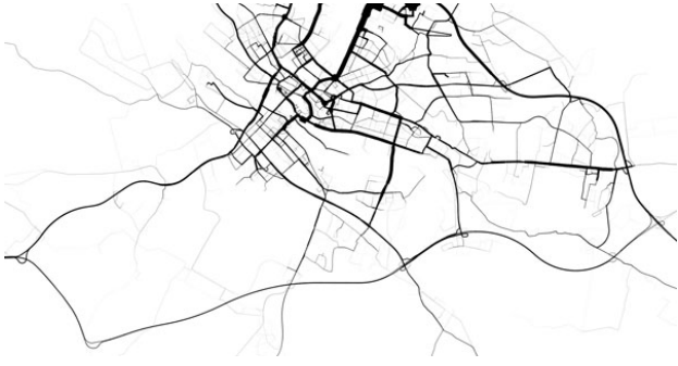
Fig. 4. Part of the road utilization map of the model region for the initial year of operation. The thickness of road segments indicates the frequency of road utilization. Map data © OpenStreetMap contributors, CC-BY-SA
