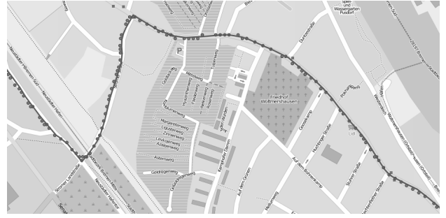
Fig. 3. Section of a trip's GPS coordinates (gray dots) mapped onto the road graph using our method (mapped edges are shown by dark gray line). © OpenStreetMap contributors, CC-BY-SA.
