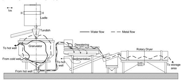
Figure 3 Typical Granshot<sup>TM</sup> set-up
