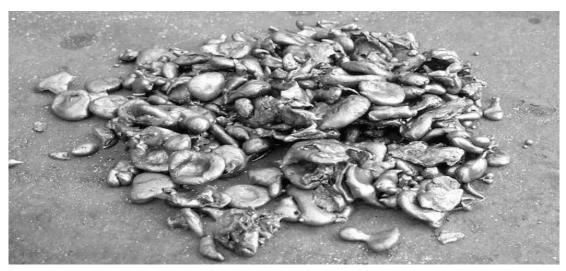
Figure 4 Granulated Pig Iron (GPITM) produced at Saldanha Steel
