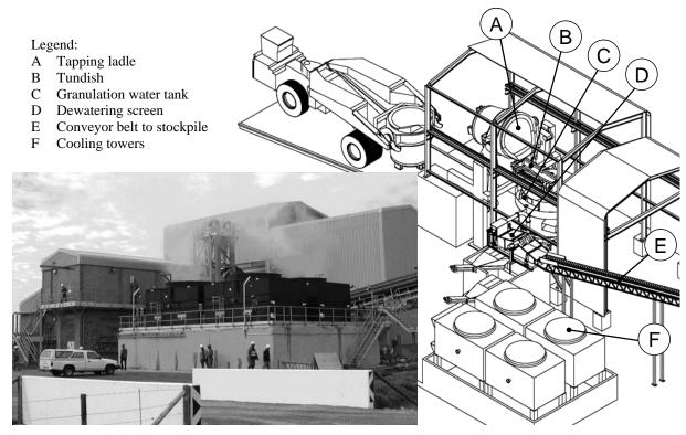
Figure 5 The Saldanha Steel granulation plant
