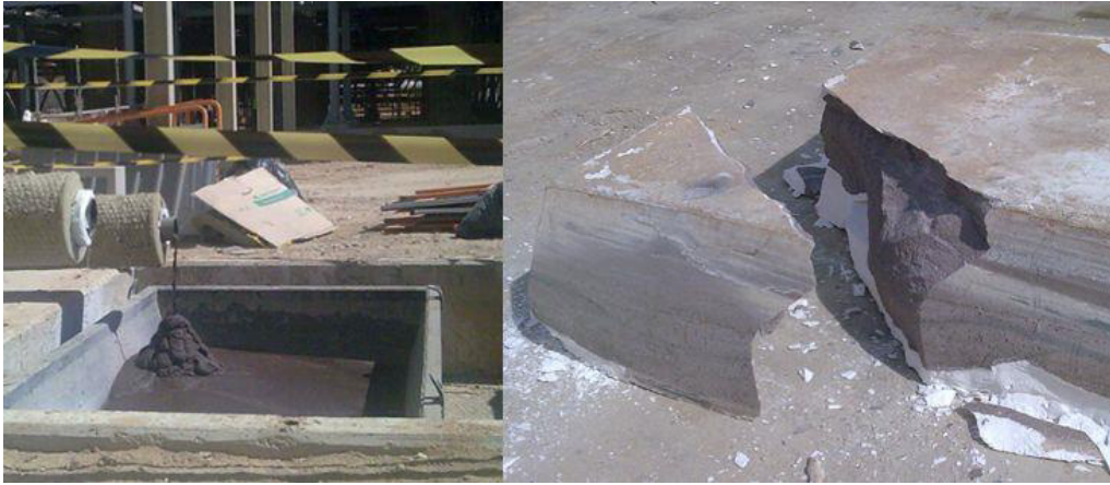
Fig. 3. Insolubles separated during initial melting process.
