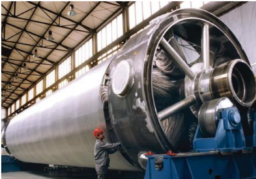
Fig. 1. CWHE tube bundle during production process and schematic drawing
