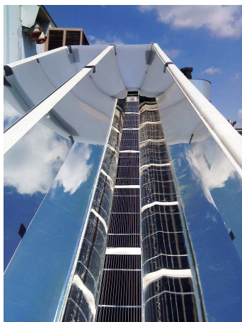
Fig. 4: PV-T CPC trough while outdoor measurement.
