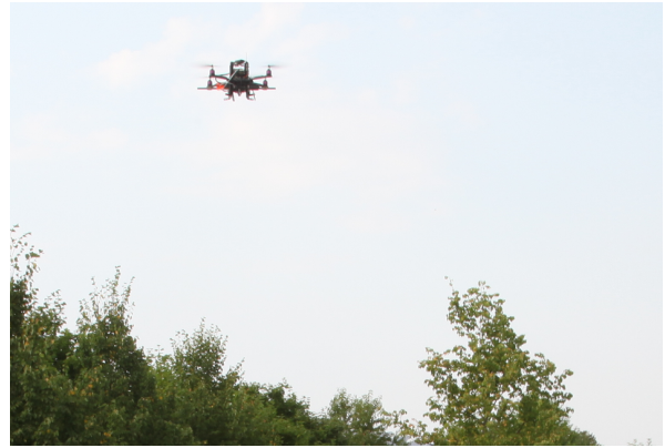
Fig. 1. Outdoor autonomous flight using only onboard IMU aided monocular vision.
