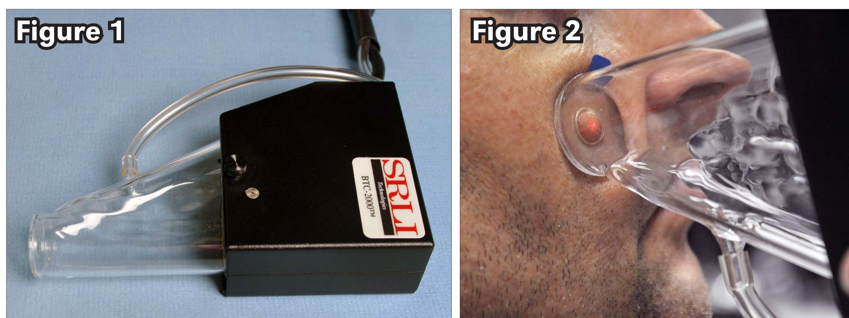
Figure 1. Glass chamber for applying vacuum to skin Figure 2. Skin being drawn into chamber with laser target on skin. Movement of laser target is detected by an infrared sensor to measure deformation.
