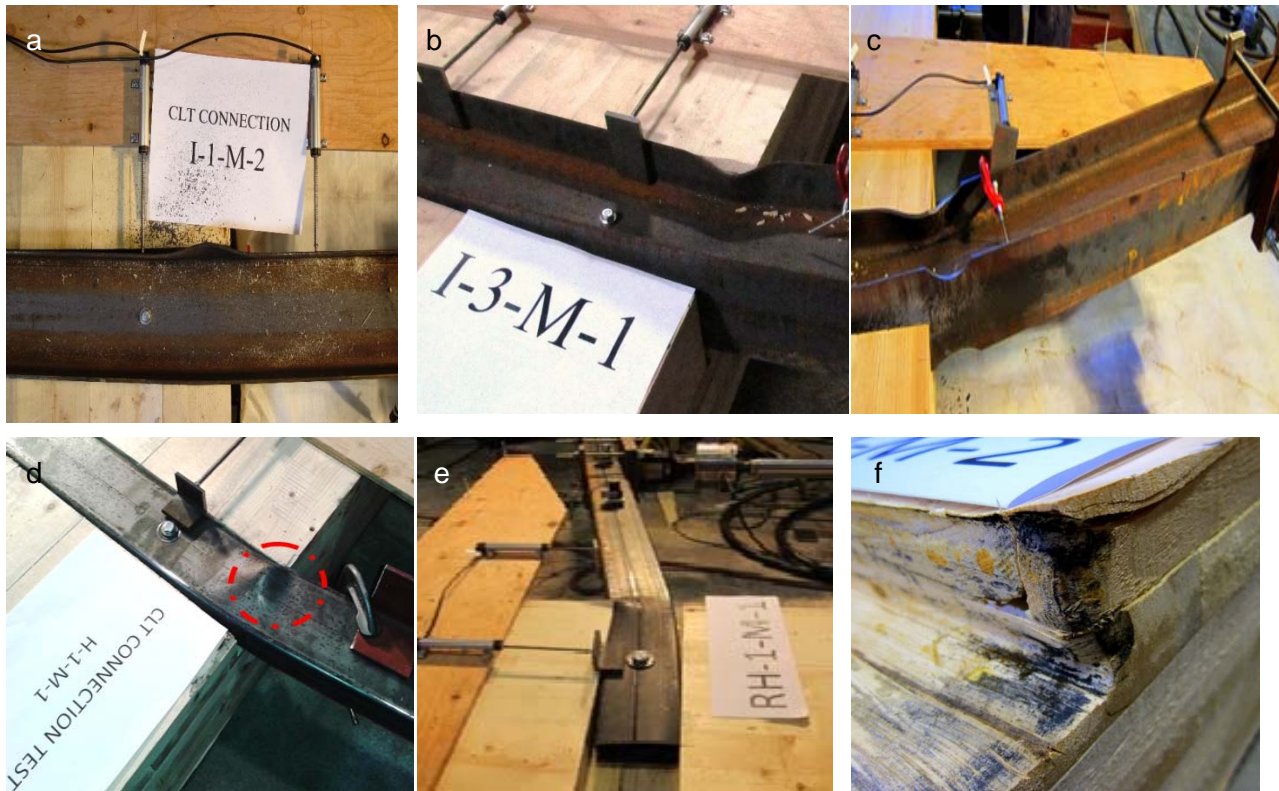
Figure 5: Test specimens after static loads: (a) Beam Yielding Series 1; (b) Beam Yielding Series 2; (c) Beam Yielding and Uplift Series 3; (d) Beam Yielding Series 4; (e) Beam Yielding Series 5; (f) Wood Damage Series 5
