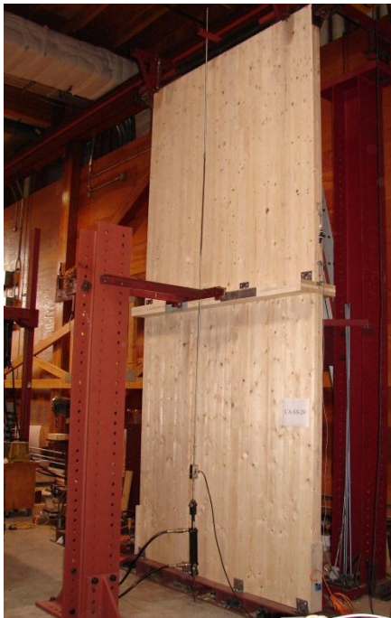
Figure 1: Two storey CLT specimen ready for testing
