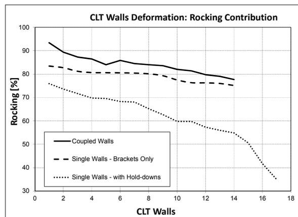
**Figure 3.2** Percentages of rocking contribution to the total CLT wall deformation at ultimate displacement under cyclic loading
