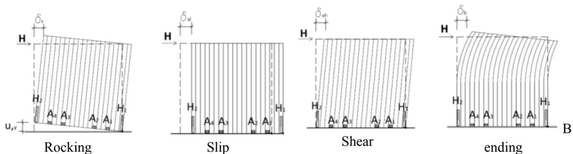
**Figure 3.1** Deflection components of a CLT wall panel (Gavric et al., 2011)
