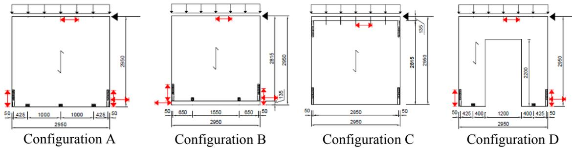
**Figure 2.1** CLT wall test configurations tested at CNR IVALSA by Ceccotti et al. (2006) (dimensions in mm)
