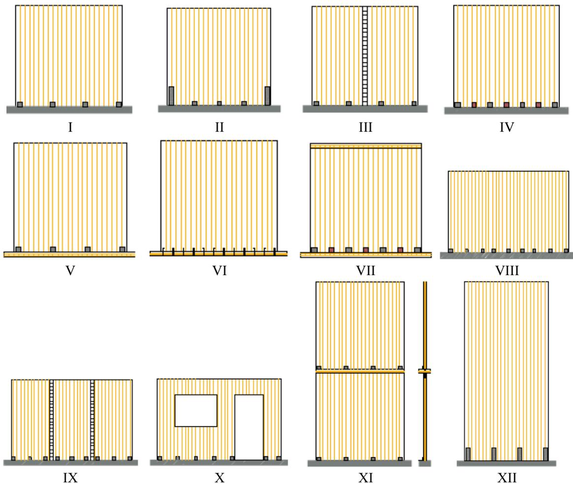
**Figure 2.3** CLT wall test configurations tested at FPInnovations by Popovski et al. (2010)
