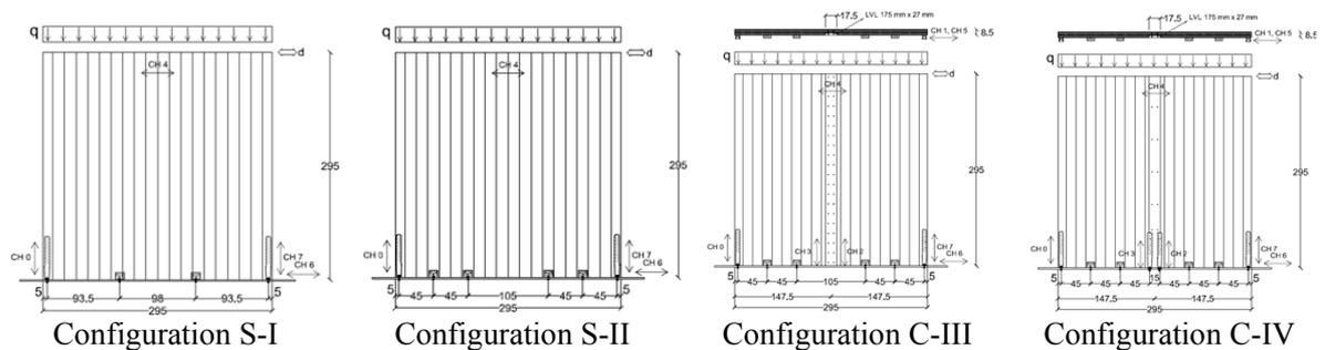
**Figure 2.2** CLT wall test configurations tested at CNR IVALSA by Gavric (2013) (dimensions in mm)
