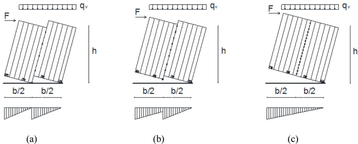
**Figure 3.3** Types of behaviour of adjacent wall panels: (a) Coupled wall behaviour; (b) Combined Single-Coupled wall behaviour; (c) Single wall behaviour
