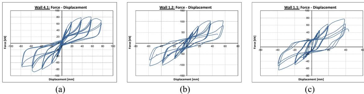
**Figure 4.1** Typical force-displacement hysteresis loops: (a) Rocking behaviour; (b) Combined Rocking-Sliding behaviour; (c) Sliding behaviour
