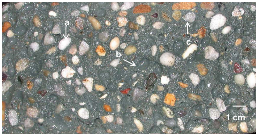
Fig. 8. Fracture surface of 50 BFS concrete with natural aggregate showing examples of: (a) unfractured stone; (b) stone pullout; and (c) fractured stone.
