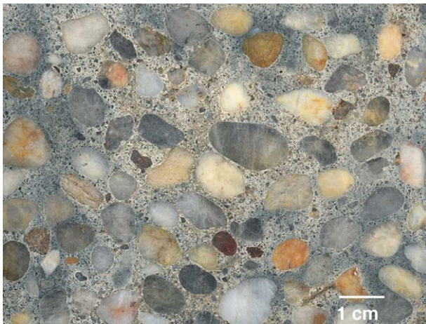
Fig. 2. Cross-section of 50 BFS concrete with 6.35–12.7 mm natural stone aggregate.
