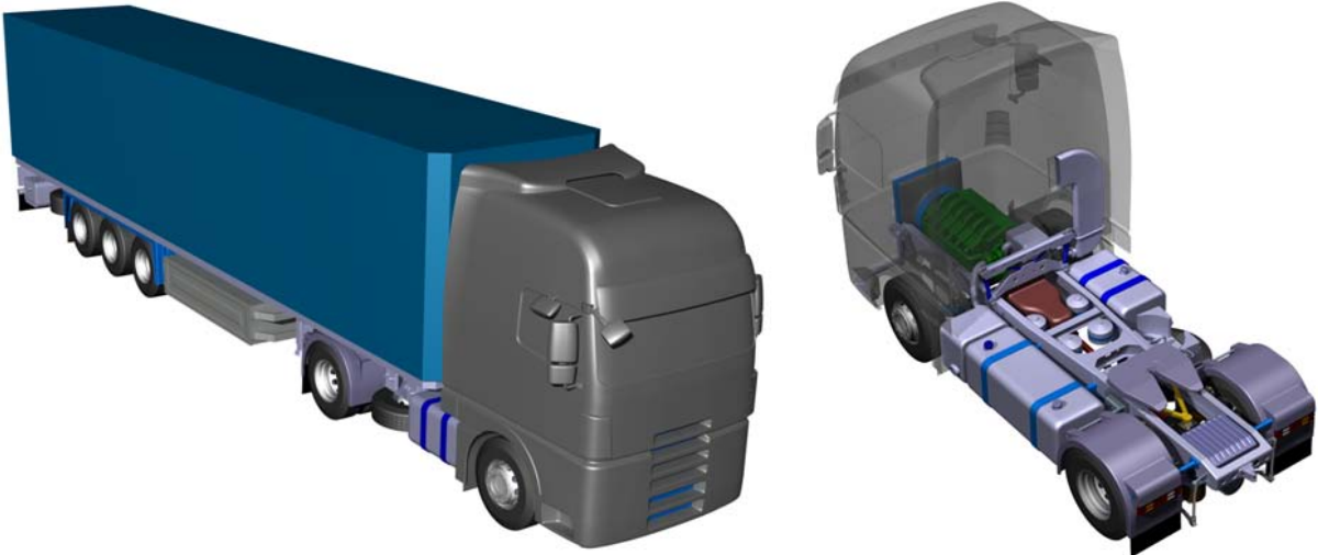
Figure 6: Detailed generic reference truck, used as a basis for the accurate aerodynamics study
