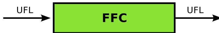
Figure 1.1: The form compiler FFC generates C++ code in UFC format from a given finite element variational form in UFL format.
