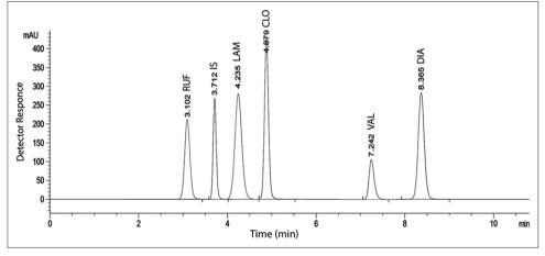
Fig. 2: High-performance liquid chromatogram of rufinamide, lamotrigine, clonazepam, diazepam, valproic acid, and lacosamide (IS) in their laboratory prepared mixture
