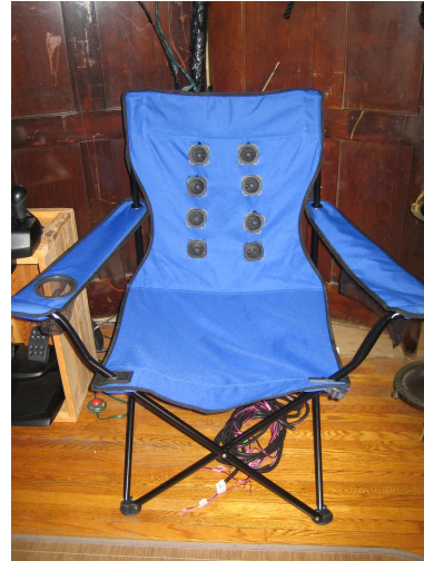
Figure 1: The MHC prototype presents 4 discrete audio-tactile channels along each of the four rows of voice coils used in the display.
