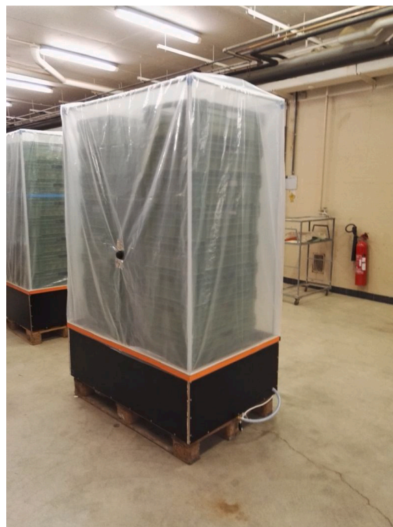
Fig. 1. Picture of one experimental chamber (0.8m × 1.2m × 2.0 m) with a total capacity of 200 kg of potatoes.
