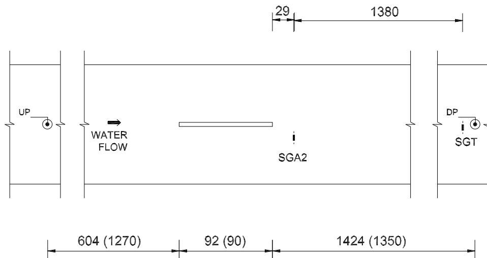
Figure 2: Location of the strain gages close to the leak (SGA2) and to the DP pressure transducer (SGT). Distances are in millimeters. Measures in brackets refer to the system with the “regular” leak (Series 2).
