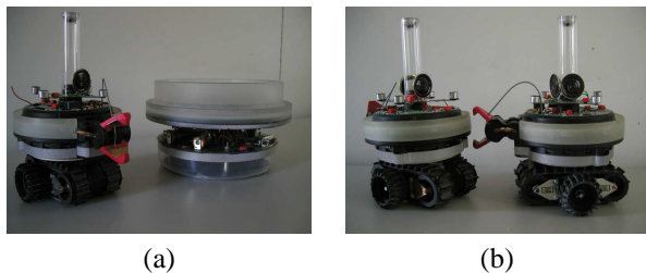
Fig. 9. A single s-bot self-assembling with (a) an object and (b) a teammate.
