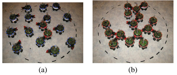
Fig. 20. Self-assembly of 16 physical s-bots put in a circle of radius 50 cm. Trial 12: (a) after 23 s and (b) after 108 s.
