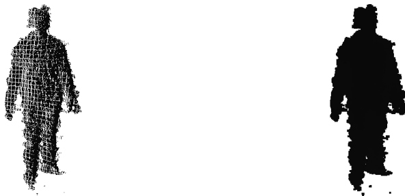
Fig. 4: On the left, the resultant point cloud re-projection to the image plane of the reference camera. On the right, the re-projection after the hole-filling procedure.
