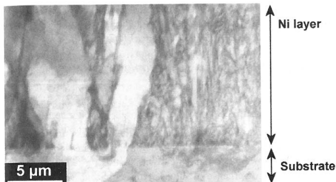
Fig. 2—TEM images of the nickel layer deposited at a current density of 3 \text{ A/dm}^2 ( 28 \text{ A/ft}^2 ) from the sulfamate bath without 1,3,6 naphthalene trisulfonic acid on the nickel substrate. The image indicates that epitaxial growth of the electrodeposited nickel can occur on certain grains of the substrate. This phenomenon was occasionally observed at the interface.
