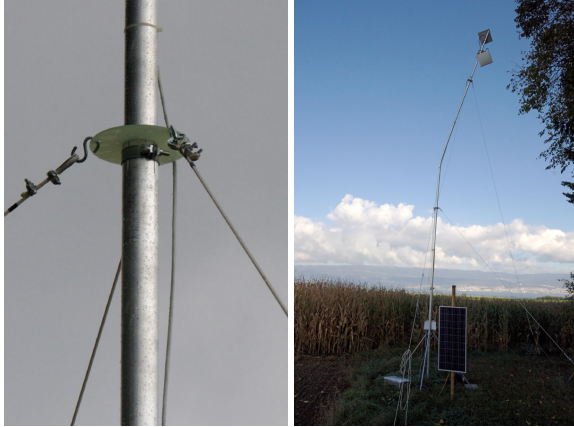
(a) Movable guying clamp to prevent torsion of mast (b) Broken antenna due to strong winds and loose guying (node02)
