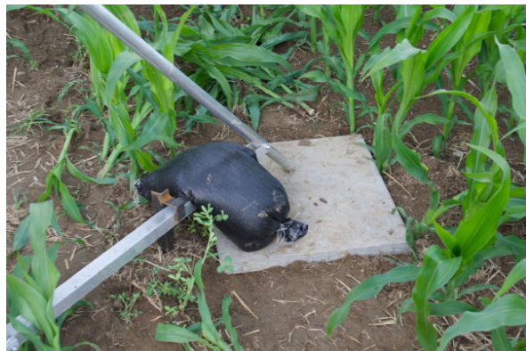
Figure 6: Concrete paving slab to prevent sinking in of the tripod, sand bag and iron stake to stabilize mast.
