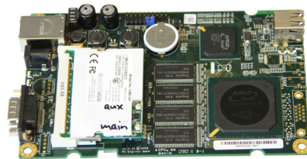
Figure 3: Mesh node: PCEngines Alix.3D board with two IEEE 802.11a/b/g/h miniPCI cards and a battery for the real-time clock.
