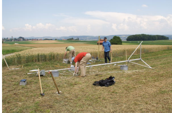
Figure 5: Complete assembly of telescopic mast in horizontal position before final setup.
