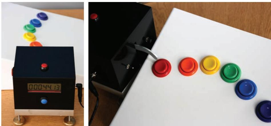
**Fig. 2.** Two views of the machine and the response box used in the machine-causal conditions of Experiments 1 and 2. The signal and target LEDs are not visible here because they were situated underneath the opaque translucent plastic cover of the box. Each LED was placed centrally above the relevant button.
