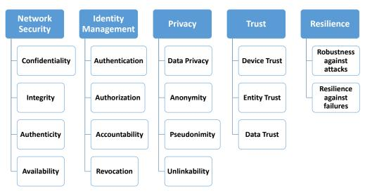
Fig. 1: Main security requirements and their subcomponents
