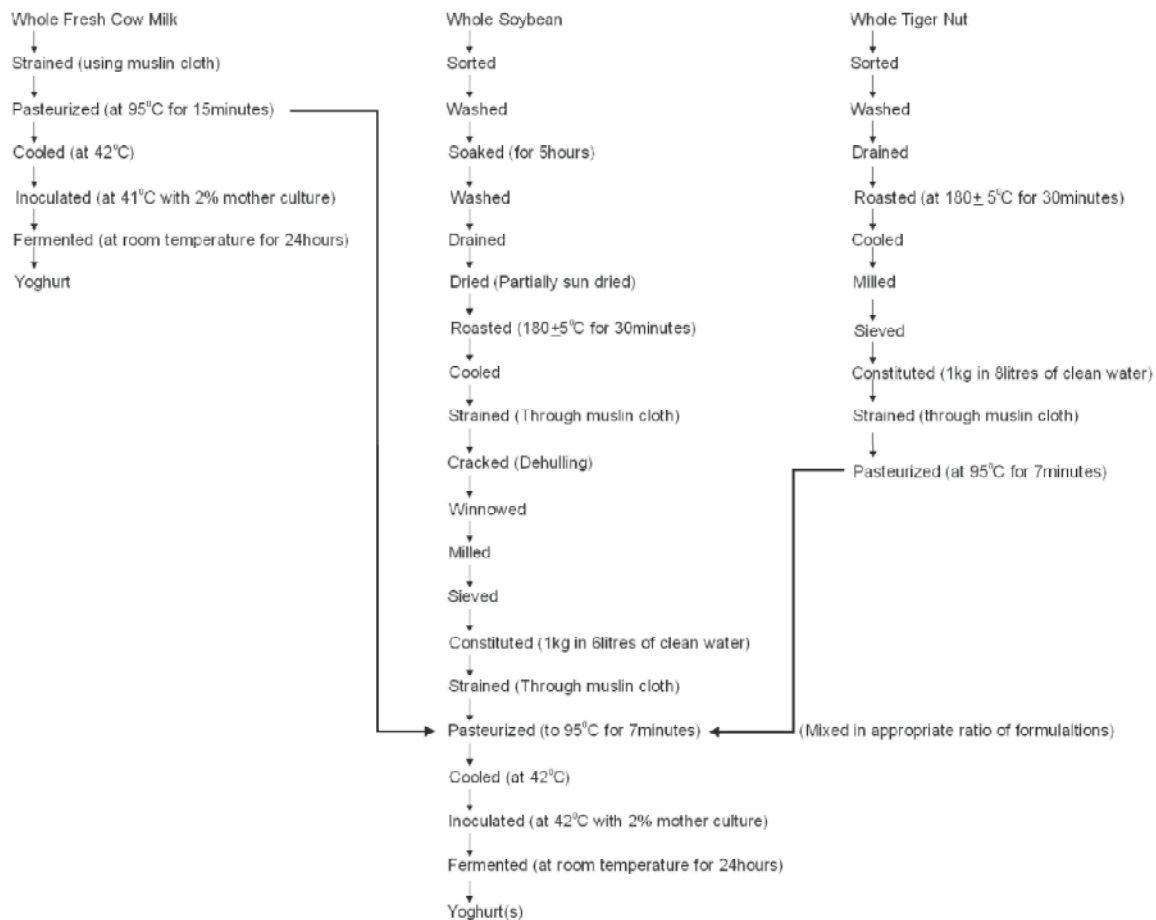
Fig. 4: Flowchart for yoghurt production Source: Adopted with modification from Bristone [32].
