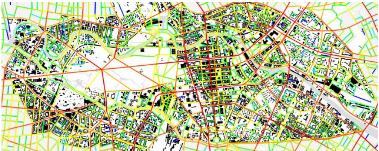
Figure 9.5 Patterns of “spatial integration” in the center of Berlin, with the highest levels of integration in red, orange and then yellow, and lower levels of integration in green, blue and then dark blue. Spatial integration measures the degree to which an urban street is connected into the overall street network Source: Rose and Schwander, 2011
