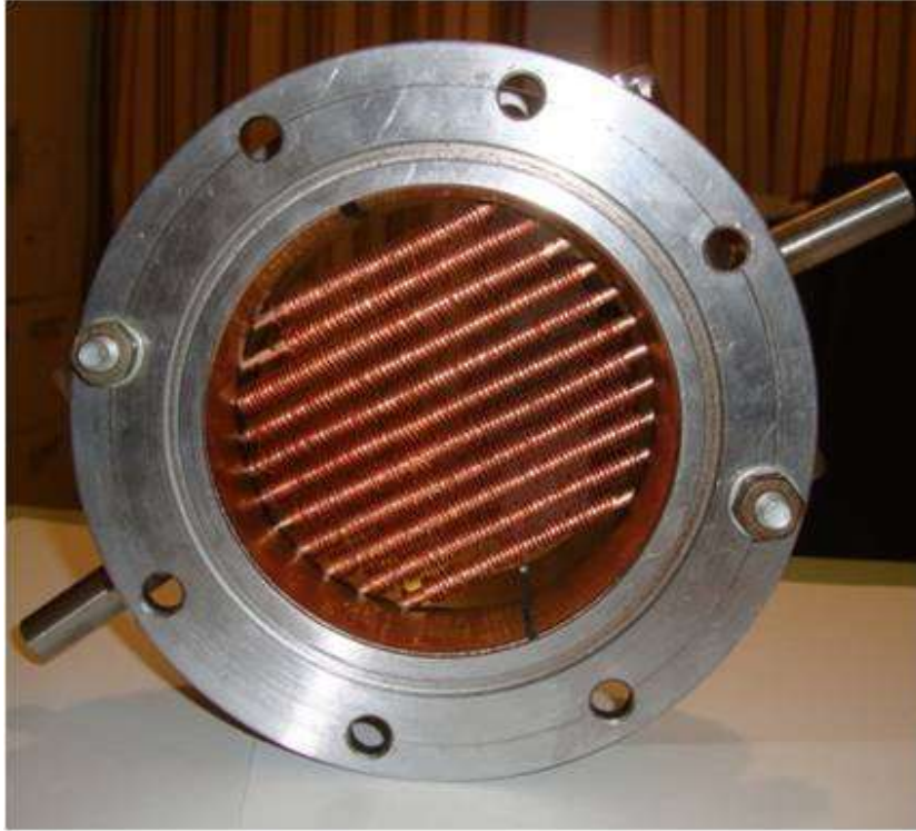
Figure 3.4: The finned tube heat exchanger inside the resonator developed specially for this study.
