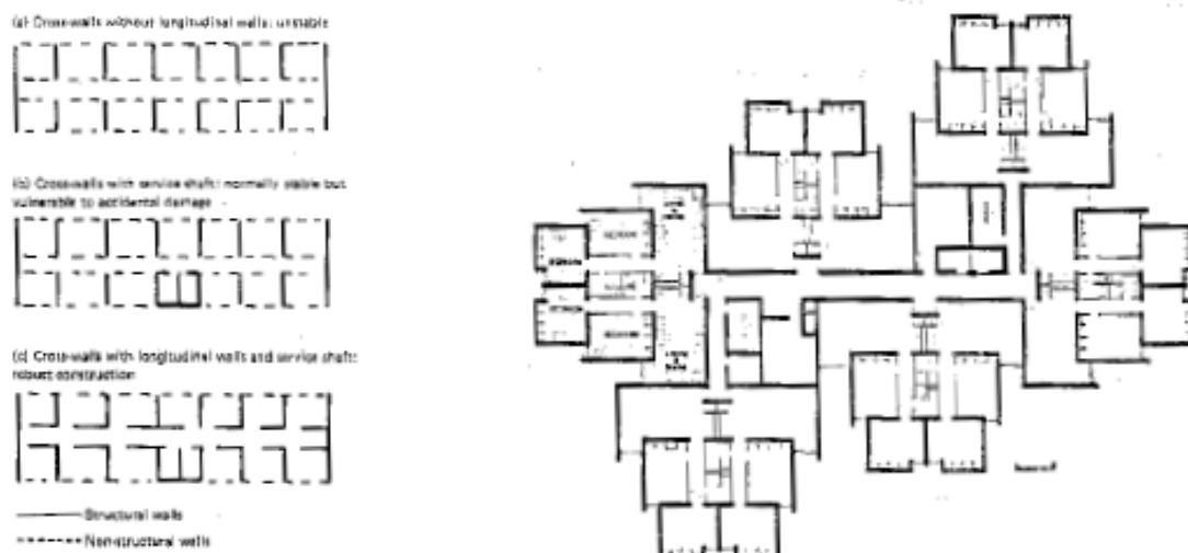
Figure 2 Suggested Layouts for Load-bearing Masonry [2]: a.
