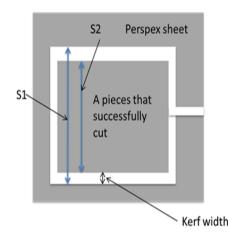
Figure 2 Schematic diagram for Kerf width measurements
