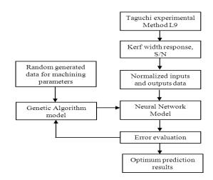
**Figure 4** A flowchart of GA-Taguchi-neural network for optimum prediction of kerf width in CO<sub>2</sub> laser cutting of Perspex
