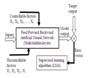
Figure 3 Computation style of ANN and Taguchi ANN-model for Laser cutting process (Training and simulation)
