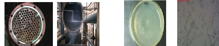
Figure-A & B. Biofouling by SRB on Heat Exchanger Figure-C Colonies of SRB Figure-D Morphology of SRB
