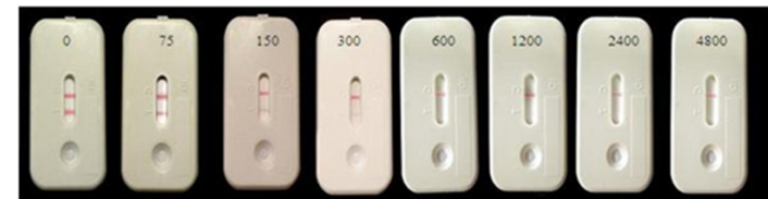
Fig. 2 A semi-quantitative competitive lateral flow device with Albugo candida zoospore numbers tested between 0 – 4800.
