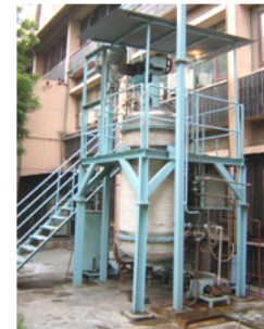
1200 L Solid- state Bioreactor: Overview & growth inside
