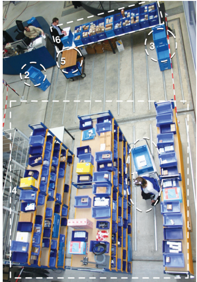
Figure 3: The warehouse with 4 shelves. The test subject wears a HMD with attached tracking markers. The WiFi-connected wireless PC is carried in a small backpack. As system control, we mounted a game show-like buzzer (adjusting knob) on the subject’s belt. The tracking is done via 6 ART DTrack1/2 Cameras.
