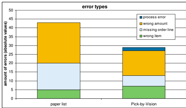
Figure 13: kinds of picking errors for both technologies before and after the correction of the systematic errors
