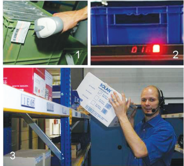
Figure 2: different common order picking technologies: MDT with scanner (1), Pick-by-Light (2) and Pick-by-Voice (3)
