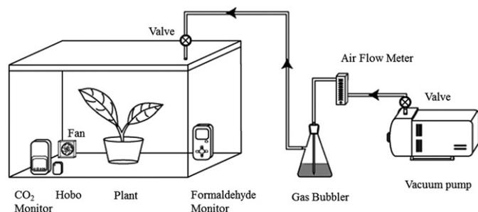
Fig. 1. Experimental setup for evaluating formaldehyde removal.
