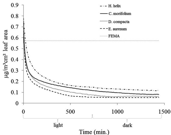
Fig. 8. Formaldehyde removal by RZ of four plant species. Initial formaldehyde concentration was  $\sim 2000 \mu\text{g m}^{-3}$  and exposure was for 24 h. FEMA: Formaldehyde levels found in bedrooms of FEMA Trailers.
