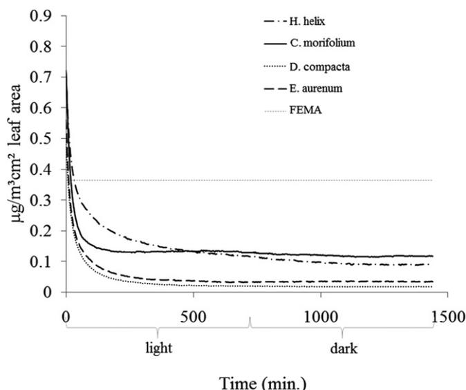
Fig. 9. Formaldehyde removal by EP of four plant species. Initial formaldehyde concentration was  $\sim 2000 \mu\text{g m}^{-3}$  and exposure was for 24 h. FEMA: Formaldehyde levels found in bedrooms of FEMA Trailers.
