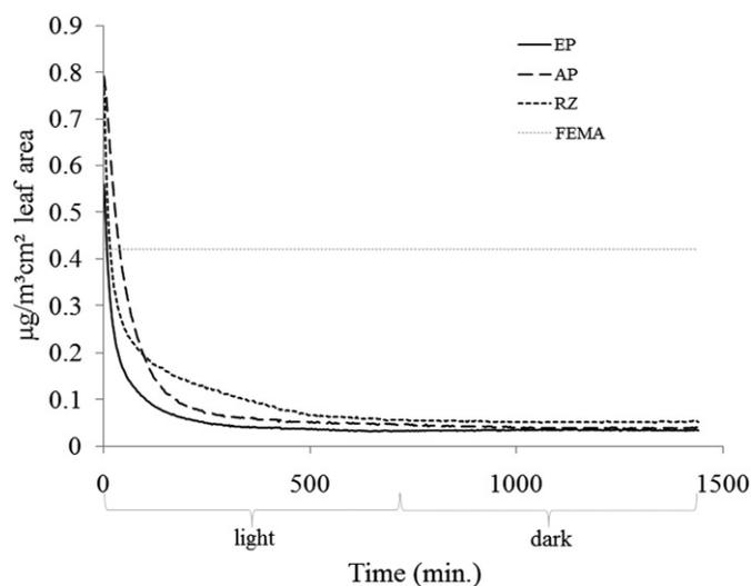
**Fig. 6.** Formaldehyde removal EP, AP parts and RZ of *E. aureum*. Initial formaldehyde concentration was  $\sim 2000 \mu\text{g m}^{-3}$  and exposure was for 24 h. FEMA: Formaldehyde levels found in bedrooms of FEMA Trailers.
