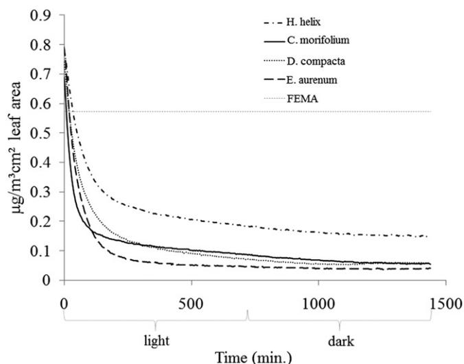
Fig. 7. Formaldehyde removal by AP parts of four plant species. Initial formaldehyde concentration was  $\sim 2000 \mu\text{g m}^{-3}$  and exposure was for 24 h. FEMA: Formaldehyde levels found in bedrooms of FEMA Trailers.
