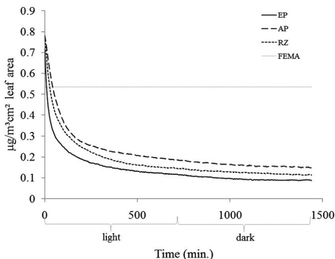
**Fig. 3.** Formaldehyde removal by EP, AP parts and RZ of *H. helix*. Initial formaldehyde concentration was  $\sim 2000 \mu\text{g m}^{-3}$  and exposure was for 24 h. FEMA: Formaldehyde levels found in bedrooms of FEMA Trailers.
