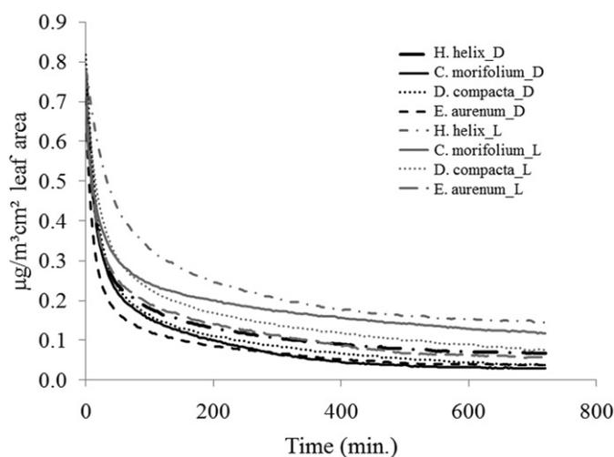
Fig. 10. Formaldehyde removal by RZ of four plant species. Initial formaldehyde concentration was  $\sim 2000 \mu\text{g m}^{-3}$  and exposure was for 24 h. FEMA: Formaldehyde levels found in bedrooms of FEMA Trailers.
