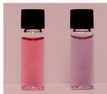
Fig. 19 LSPR detection based on ligand-induced gold nanoparticle aggregation. The resulting color change can be seen with the naked eye. (I) shows TEM images of aggregation while (II) shows resulting color change of sample solution. (a) Without cholera toxin. (b) With cholera toxin. Reprinted from ref. 86 with permission from the American Chemical Society.
