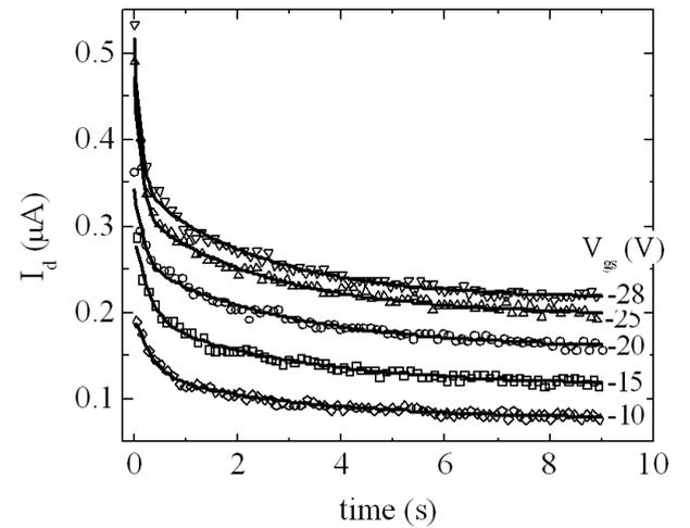
Fig. 6. Time dependence of the drain current (symbols) of a pentacene TFT measured in air after a gate voltage is applied at various gate voltages.  $I_d$  curves are fitted by using a two-exponential-decay function (solid lines).
