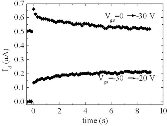
Fig. 7. Time dependence of the drain current of a pentacene TFT measured in air after a  $V_{gs} = -30$  is applied (diamonds) and after changing  $V_{gs}$  from  $-30$  V to  $-20$  V (circles).
