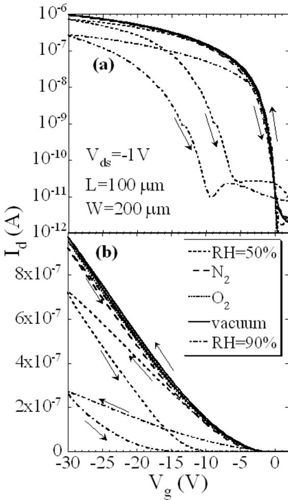
Fig. 1. (a) Semilogarithmic and (b) linear plots of transfer characteristics of pentacene TFTs measured under different environmental conditions.
