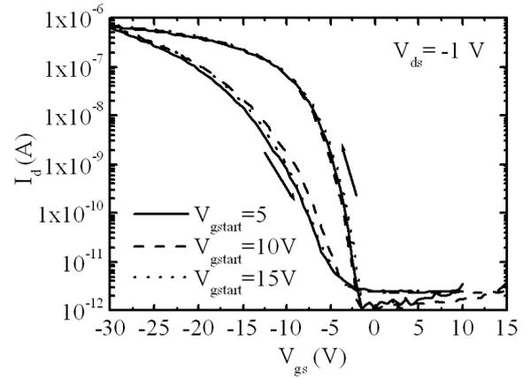
Fig. 2. Transfer characteristics of pentacene TFTs measured in air with different starting gate voltages.
