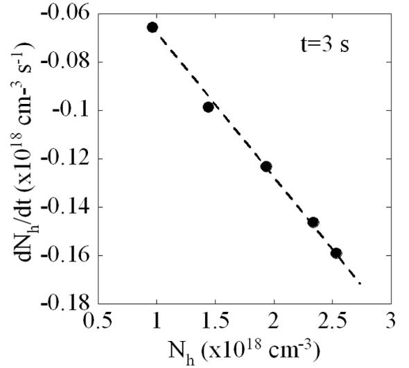
Fig. 8. The rate of decrease of the hole concentration,  $dN_h/dt$ , plotted versus the hole concentration,  $N_h$ , measured at constant time ( $t = 3$  s) and various  $V_{gs}$ .  $dN_h/dt$  and  $N_h$  were calculated from the data shown in Figure 6.
