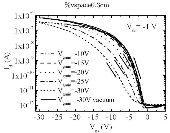
Fig. 3. Transfer characteristics of pentacene TFTs measured in air with different lower gate voltages.
