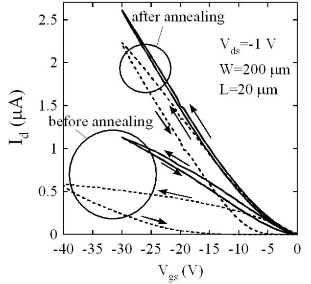
Fig. 5. Transfer characteristics of pentacene TFTs with a parylene passivation layer measured in vacuum (solid lines) and in air (dashed lines) before and after thermal annealing.
