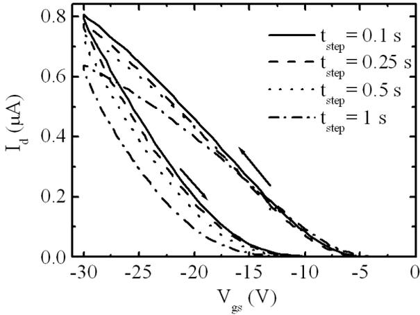
Fig. 4. Transfer characteristics of pentacene TFTs measured in air with different ramp rates.
