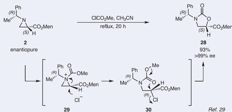
Scheme 8. Ring Expansion of Aziridine-2-carboxylate **2** into the Corresponding Oxazolidinone.
