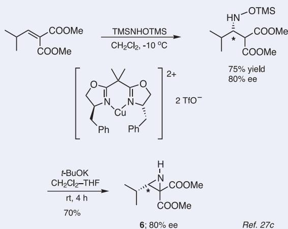
**Scheme 7.** Synthesis of Aziridine-2,2-dicarboxylates by a 1,4-Addition Reaction.
