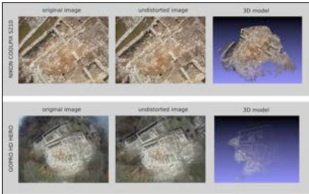
**Figure 6.** Comparison between the two cameras: original picture, undistorted image, 3D point cloud.
