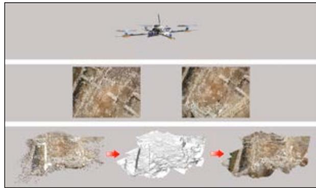
**Figure 7.** The data processing: from the original pictures to the final 3D model (point cloud, mesh, texture).
