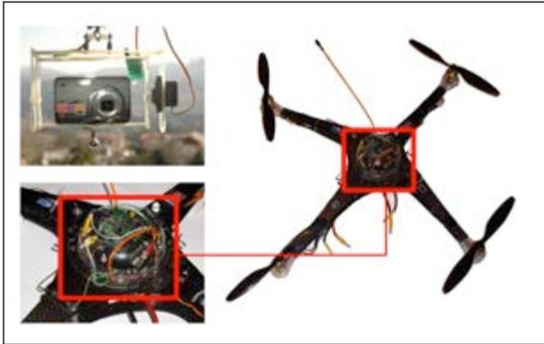
**Figure 2.** three images of the UAVP drone built by Arc-Team: the remote sensing device (up-left), the motherboard (down-left) and the quadcopter (right).
