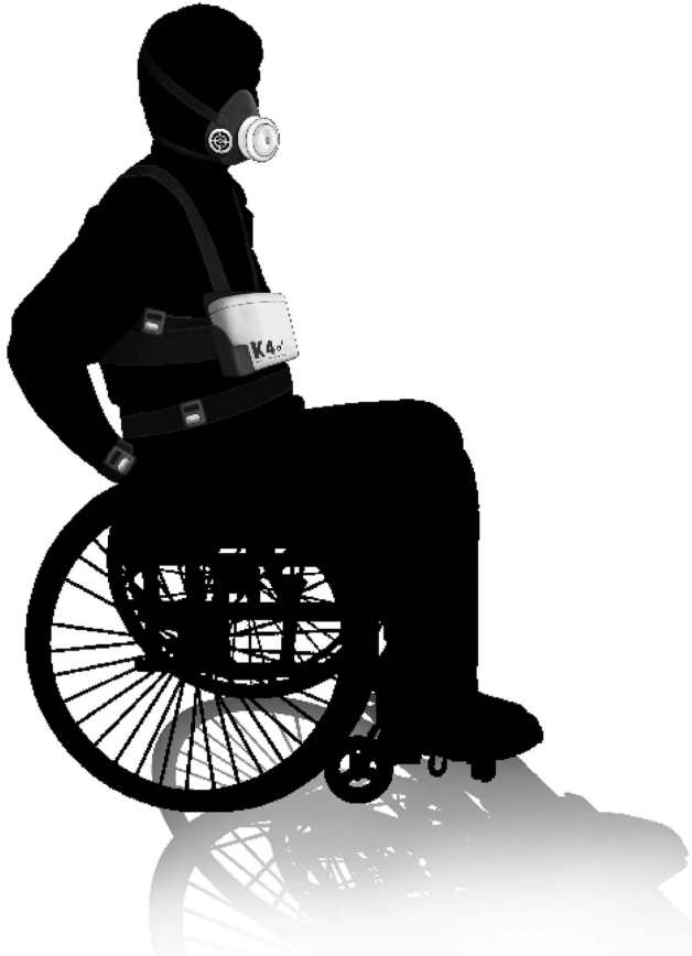
Figure 1 Instrumentation set-up. The individual wear four accelerometers: one on each wrist, one on the waist and one in the chest. Further, the portable gas analysis system is placed with a harness on the chest and connected to the mask, placed over the mouth and nose.
