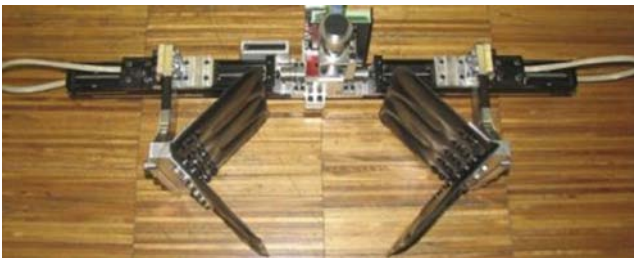
Figure 14 Gripper of the 3DCLIMBER robot
