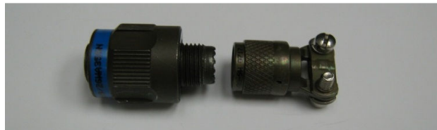
Fig. 1 D38999 Connector with Standard Backshell
