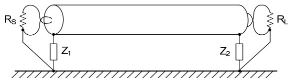
Fig. 8 Shield Termination Impedances for Twisted Shielded Pair
