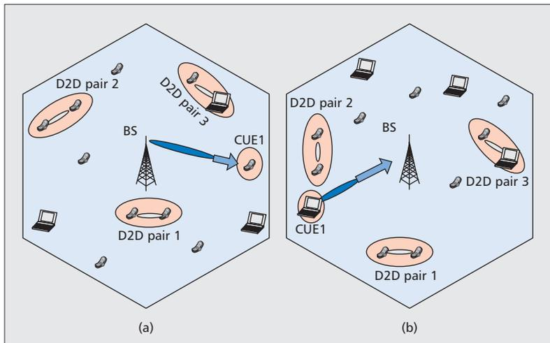
Figure 4. MmWave transmission in non-orthogonal D2D communications.
