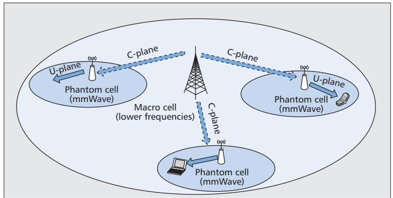
Figure 5. MmWave small cells with C-plane/U-plane split.
