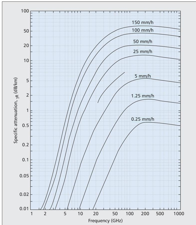
**Figure 1.** Rain attenuation in dB/km at various rainfall rates (figure from [8]).
