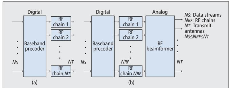
Figure 2. Beamforming diagrams: a) sub 3 GHz system; b) mmWave system.
