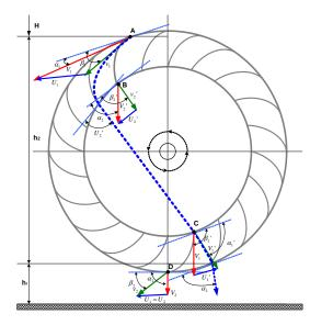
Fig.1. Path of water through turbine<sup>[11]</sup>
