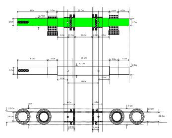
Fig. 9. Design shaft of the new micro turbine
