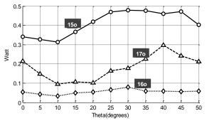
Fig. 13. Power output of the water wheel vs nozzle angle  $\theta$
