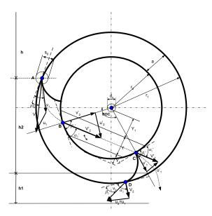
Fig. 6. Path of jet inside wheel <sup>[11]</sup>
