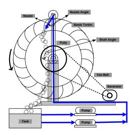
Fig. 10. Design model simulation of the micro turbine
