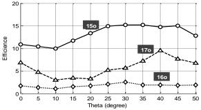
**Fig. 12.** Efficiency of the relative water wheel nozzle angle  $\theta$
