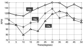
**Fig. 14.** RPM of the water wheel vs the nozzle angle  $\theta$
