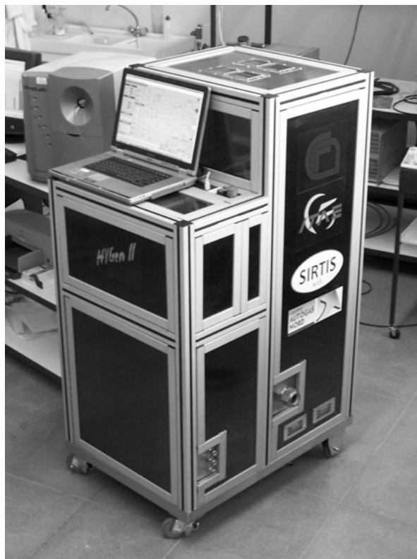
Figure 1. View of the 5 kWeq fuel processor (HYGen II).
