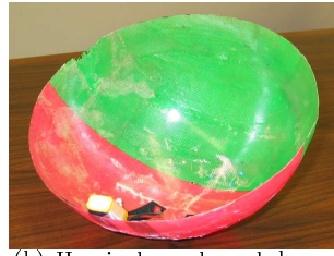
(b) Hemisphere-shaped drogue with 30 cm diameter made of reinforced plastic.
