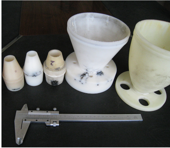
FIG. 1. Photo of the failed insulators due to bulk breakdown under sub-nanosecond pulses with pulse width of 0.6 ns.
