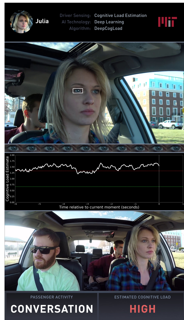
Figure 1: Illustrative example of real-time cognitive load estimation during active conversation between driver and passenger. Videos of real-time cognitive load estimation in various contexts (including outside the driving context) are available on https://hcai.mit.edu/cognitive . This visualization shows (1) the video of the driver’s face, (2) the 10 recent snapshots of the eye region, (3) the 30Hz cognitive load estimation plot, (4) the video of the cabin, and (5) the estimated class of cognitive load.
