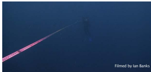
Figure 6 Visibility Measurement using Secchi disk with diver and Secchi disk just visible.
