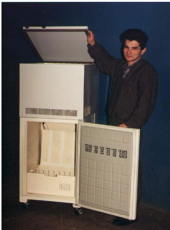
Fig. 25. Solid sorption refrigerator (lower part) and drying chamber (upper part) [10] with heat pipe thermal control. Refrigerator cooling capacity is 200 W.
